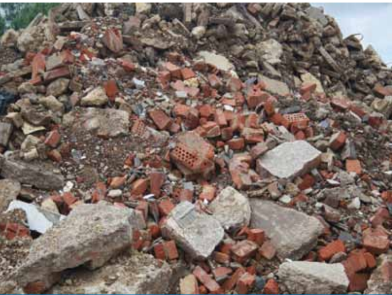
Construction & Demolition Waste Feed Material
