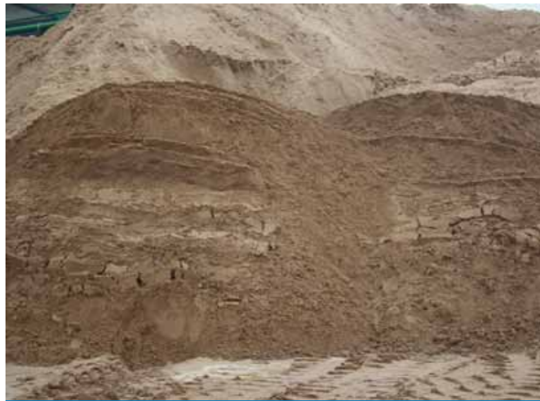
Recycled Sand Stockpile
